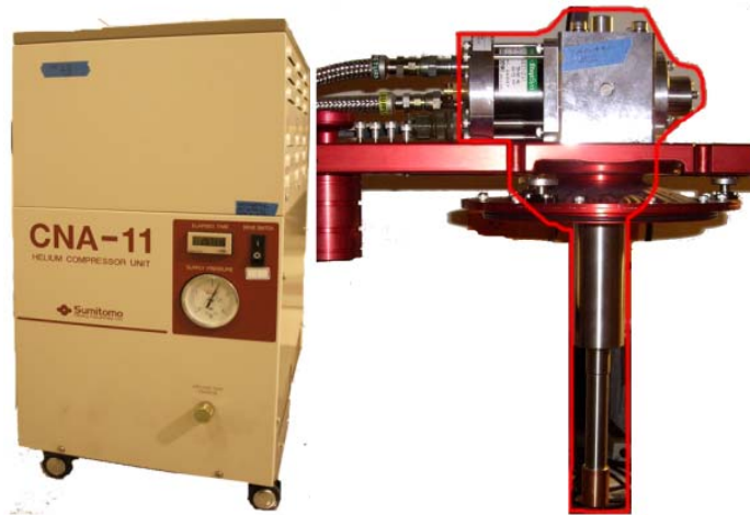
Fig. 2-3 Refrigeration system of Sumitomo CNA-11 helium compressor, and Sumitomo RDK-101E coldhead of T48
