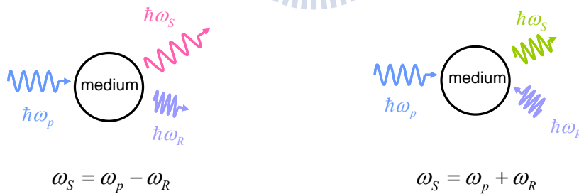
Fig. 2-1. Spontaneous Raman scattering with (a) Stokes photon generation ( \omega_S < \omega_p ) and (b) anti-Stokes photon generation ( \omega_S > \omega_p )
