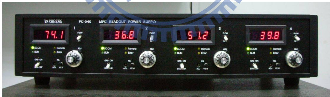
Figure III.2. PC-540 Four-channel MFC readout power supply.
