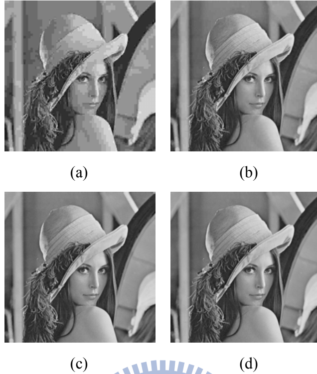
Figure 3.5. Four versions of the important image Lena reconstructed from various numbers of received JPEG stego codes: (a) from any three JPEG stego codes (PSNR=27.32 dB); (b) from any four JPEG stego codes (PSNR=33.67 dB); (c) from any five JPEG stego codes (PSNR=39.35 dB); (d) from the six JPEG stego codes (and identical to the original important image Lena).
