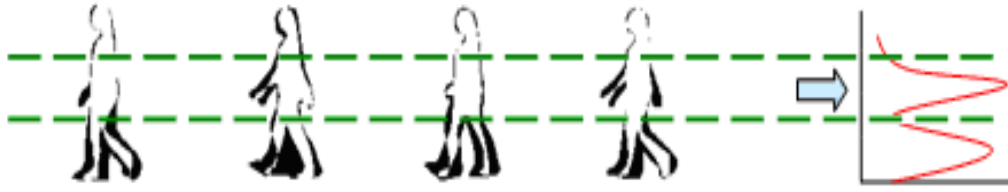
Figure 2.11 The constituent components of a posture are partitioned based on local variance extraction. The dashed lines which separate postures into constituent components are determined based on the distribution of local variance shown on the right-hand side.
