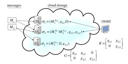
Figure 3.1: A storage system using the random erasure code. Messages  $M_1$  and  $M_2$  are randomly distributed to storage servers  $SS_1$ ,  $SS_2$ , and  $SS_3$ . The storage server  $SS_1$  randomly selects a coefficient  $g_{1,1}$  for the received message. Similarly, the storage servers  $SS_2$  and  $SS_3$  individually select coefficients.
