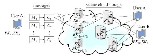
Figure 3.3: The advanced system model of our secure cloud storage system. User A generates a re-encryption key  $\mathsf{RK}_{A\to B,\mathsf{F}_{id}}$  and distributes it to all storage servers such that the storage servers re-encrypt the ciphertexts into ones under user B's key.
