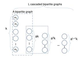
Figure 2.10: The encoding structure of Tornado codes.
