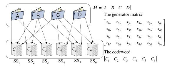
Figure 2.12: A networked storage system using a random linear code. Each storage server selects a random coefficient for each received message. The linear combination is performed by the storage server. Each column of the generator matrix and each codeword symbol is determined and computed by a storage server. No central authority is required in the encoding process.
