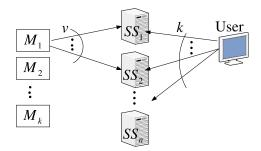
Figure 2.13: A networked storage system using a decentralized erasure code. The settings for the parameters n, k, and v and the random process of data distribution determine the probability of a successful data retrieval.
