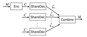
Figure 4.2: The flowchart of the threshold encryption scheme. The flow of encryption and partial decryption of the threshold encryption scheme. Message M is encrypted as C. The decryption is performed by m partial decryption processes and a final combine process.
