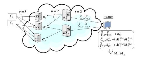
Figure 4.4: A storage system using the secure decentralized erasure code.
