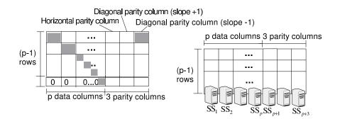
Figure 2.8: The STAR encoding and a system storing the encoded data. STAR codes tolerate the failure of 3 servers. There are 3 columns of parity bits.
