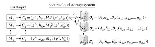
Figure 4.3: The storage process of our first secure cloud storage system. The messages are encrypted and distributed among the storage servers. Each storage server combines all received ciphertexts and stores the result and the chosen coefficients.
