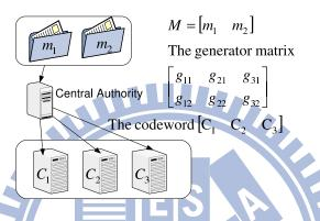
Figure 2.5: An example of a storage system that uses a linear code. The central authority encodes the messages into a codeword  $(C_1, C_2, C_3)$  and sends a distinct symbol to a storage server for storage.
