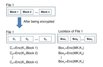
Figure 2.15: File 1 before and after being encrypted in a Plutus system. The file is divided into blocks and each file block is encrypted by using a distinct symmetric key. All symmetric keys are encrypted by using another symmetric key MK. The encrypted symmetric keys are stored with the encrypted file blocks. A user may use a different MK for each file.
