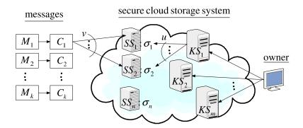
Figure 3.2: Our first system model of our secure cloud storage system. Messages are encrypted and then randomly distributed amon the storage servers. Each storage server performs the combination on received ciphertexts and only stores the result and chosen coefficients.
