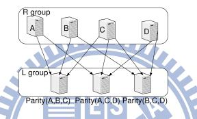
Figure 2.9: A networked storage system that uses a LDPC code. The system contains 7 storage servers and 4 out of them store the original data. The other 3 storage server store the parity results of the data.
