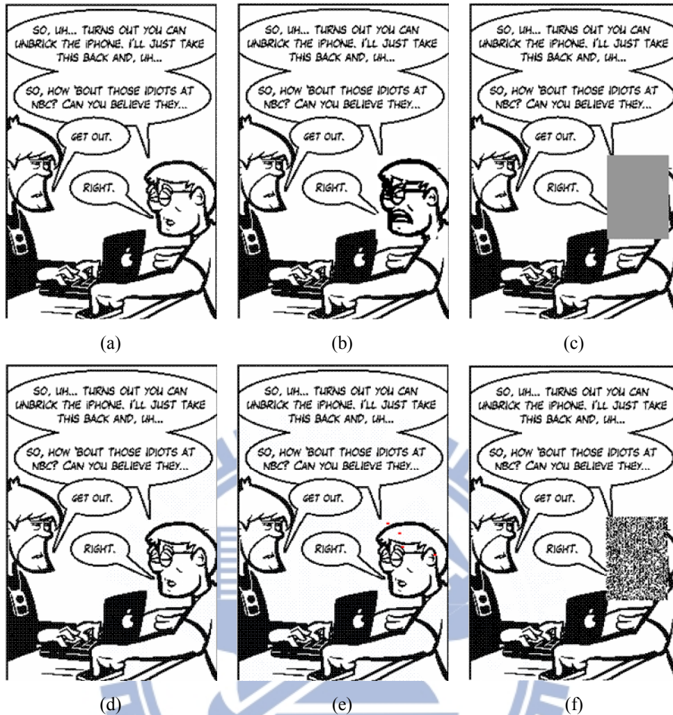
Fig. 4.4 Another authentication result of a stego-image of comic attacked by the superimposing operation. (a) A stego-image. (b) Tampered image yielded by superimposing a fake face on the person at the right side in Fig. 4.4(a). (c) Result with tampered blocks detected and marked as gray. (d) Result of image recovery. (e) Result of image recovery with red dots indicating unrecovered tampered blocks. (f) Erroneous image recovery result obtained with a wrong key.
