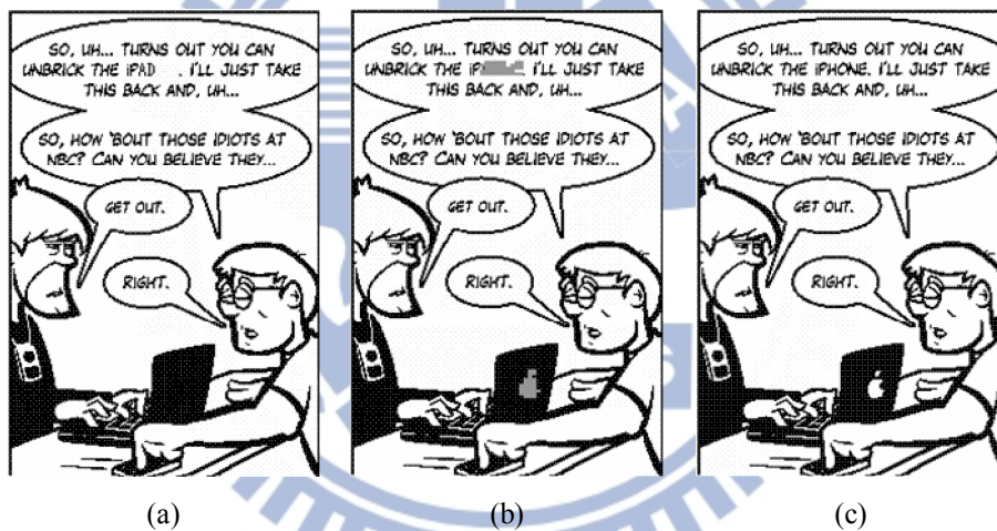
Fig. 4.6 Authentication result of a stego-image of comic attacked by painting. (a) A tampered image. (b) Result of authentication with tampered blocks detected and marked as gray. (c) Result of image recovery.
