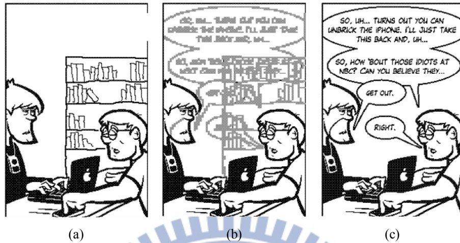
Fig. 4.7 Authentication results of a stego-image of comic attacked by painting. (a) A tampered image. (b) Result of authentication with tampered blocks detected and marked as gray. (c) Result of image recovery.
