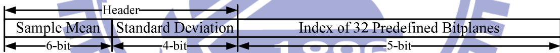
Fig. 8 Compressed 16-bit segment format of Block Truncation Coding using a set of predefined bitplanes
