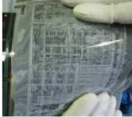
Gate-driver-integrated 15" WXGA AM-LCD 1280×720 (SEC, 2008)
