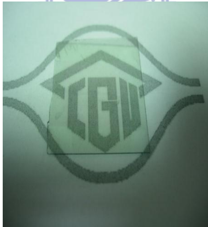
Fig. 4-19 The logo under this transparent ITO/Gd 2 O 3 /ITO structure is clearly been seen.
