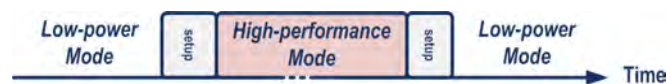
Figure 5.2: A wireless sensor node with two operating modes: Low-power Mode and High-performance Mode .
