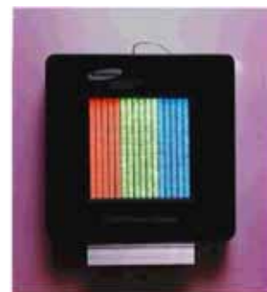
Fig. 1.4 (a) Sony portable DVD player using a Candescent field emission display [16], (b) Motorola 15 inch field emission display [16], (c) Motorola 5.6 inch color FED, (d) Pixtech 5.6 inch color FED, (e) Futaba 7 inch color FED, and (f) 7 inch color CNT FED from Samsung .
