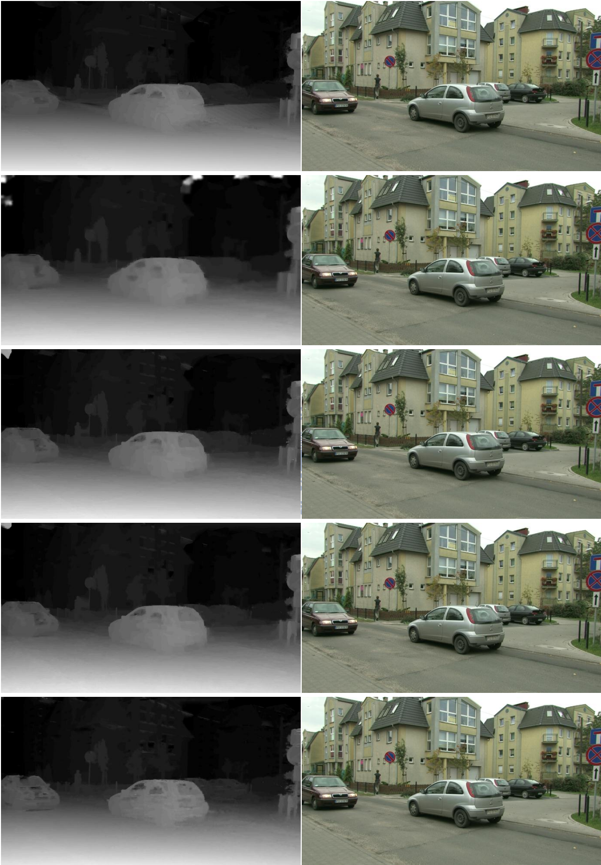
Figure V-15 Disparity maps and view synthesized images in the 167 th frame of CarPark Results from top to down are by the DERS, baseline, HQ-DE, SC-DE, HE-DE algorithms.
