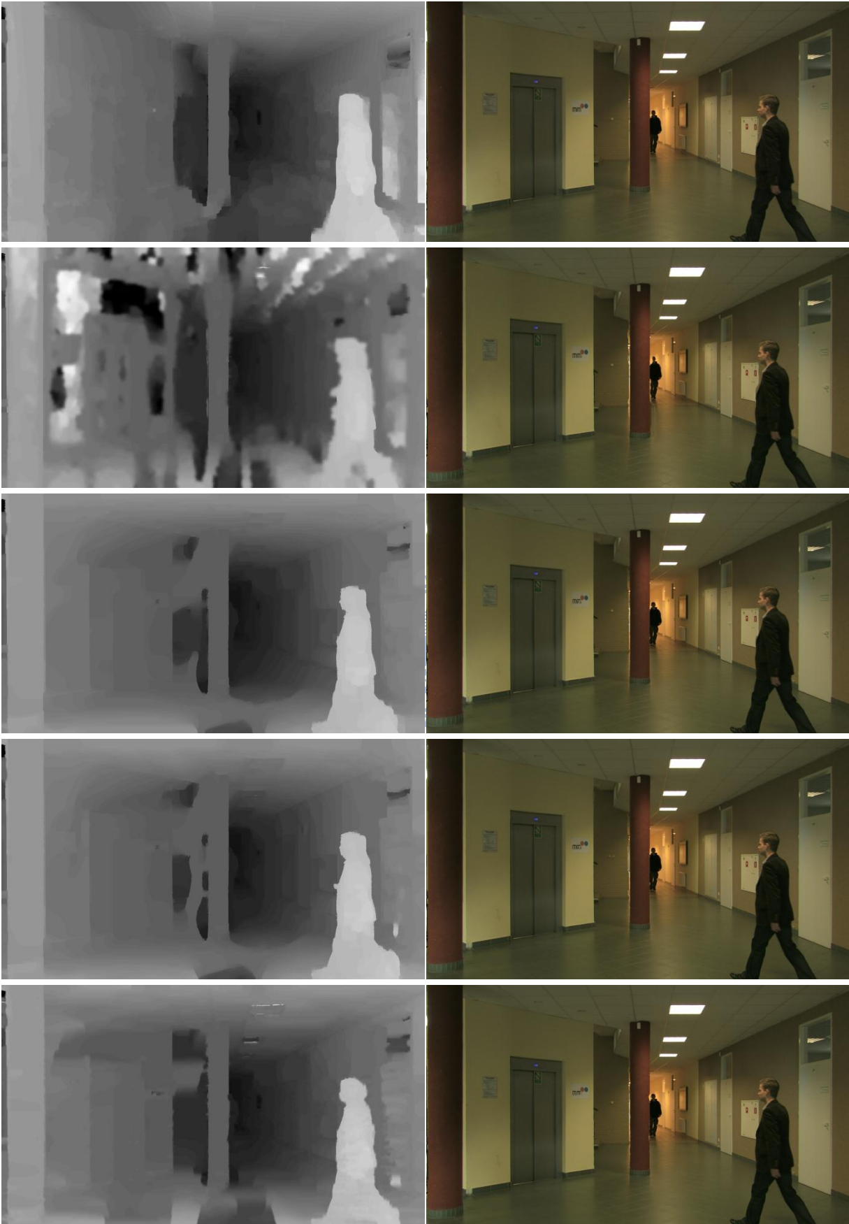
Figure V-13 Disparity maps and view synthesized images in the 50 th frame of Hall1 Results from top to down are by the DERS, baseline, HQ-DE, SC-DE, HE-DE algorithms.
