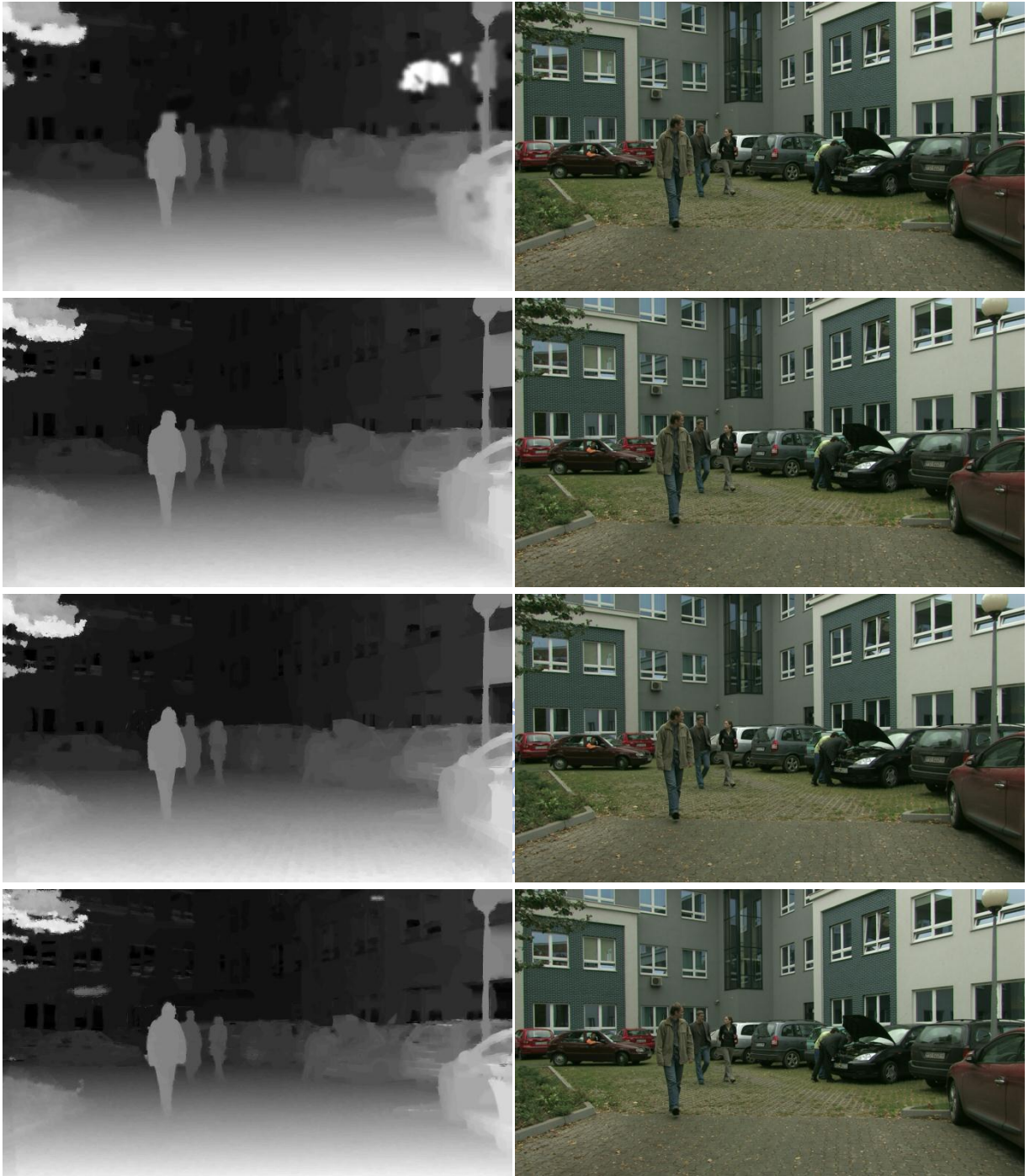
Figure V-16 Disparity maps and view synthesized images in the 50 th frame of CarPark Results from top to down are the produced by the baseline, HQ-DE, SC-DE, HE-DE algorithms.
