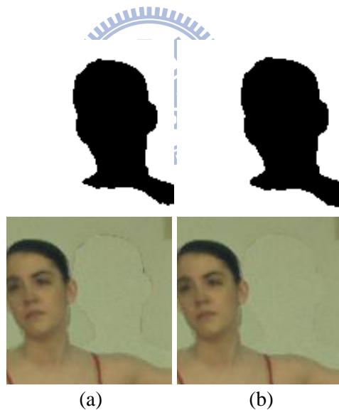
Figure II-14 Blending step in view synthesis (a) without hole dilation, (b) with hole dilation
