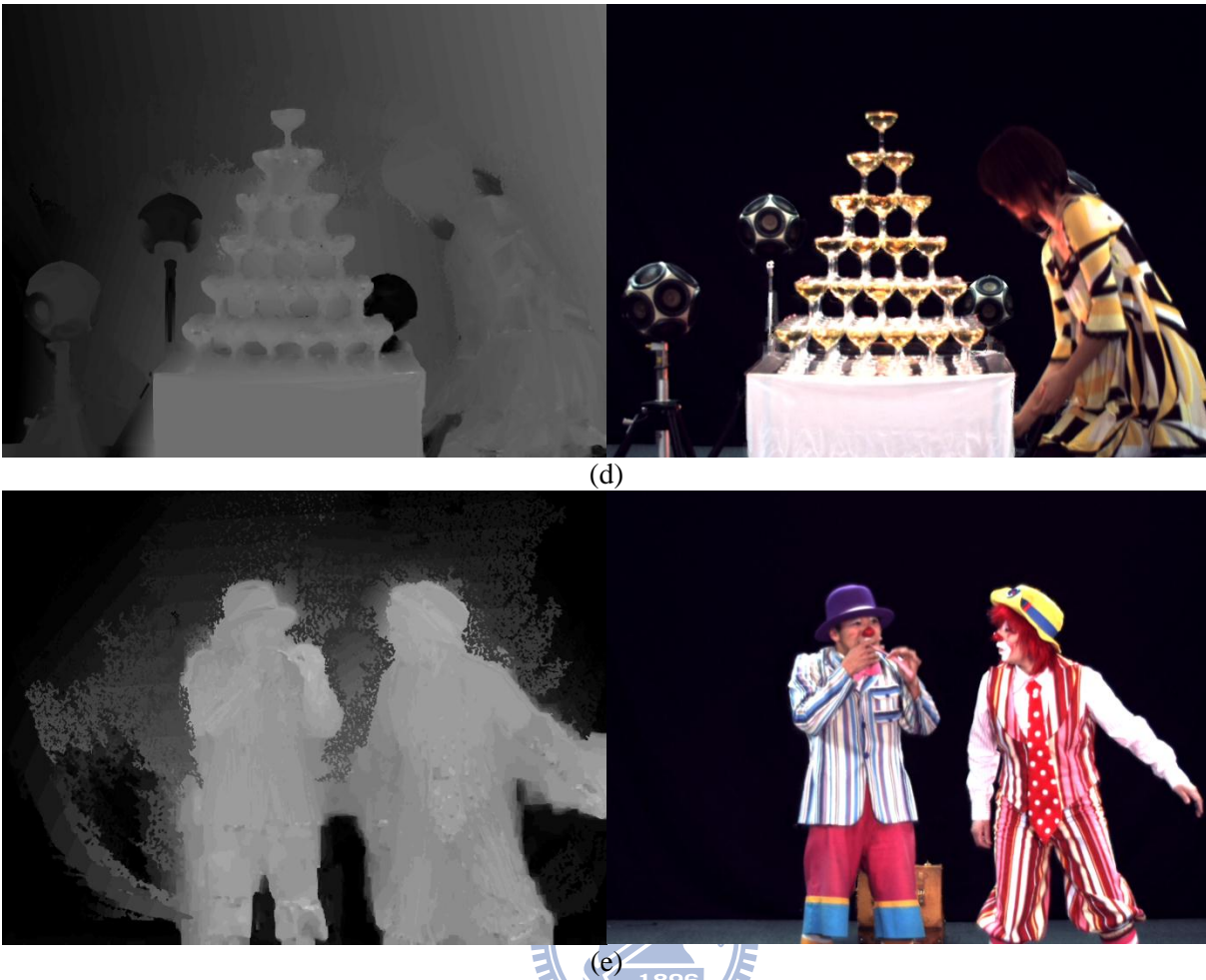
Figure III-29 Center disparity maps and synthesized View8 of DERS algorithm at the 100th frame (a) BookArrival, (b) LoveBird1, (c) Newspaper, (d) Champagne, (e) Pantomime
