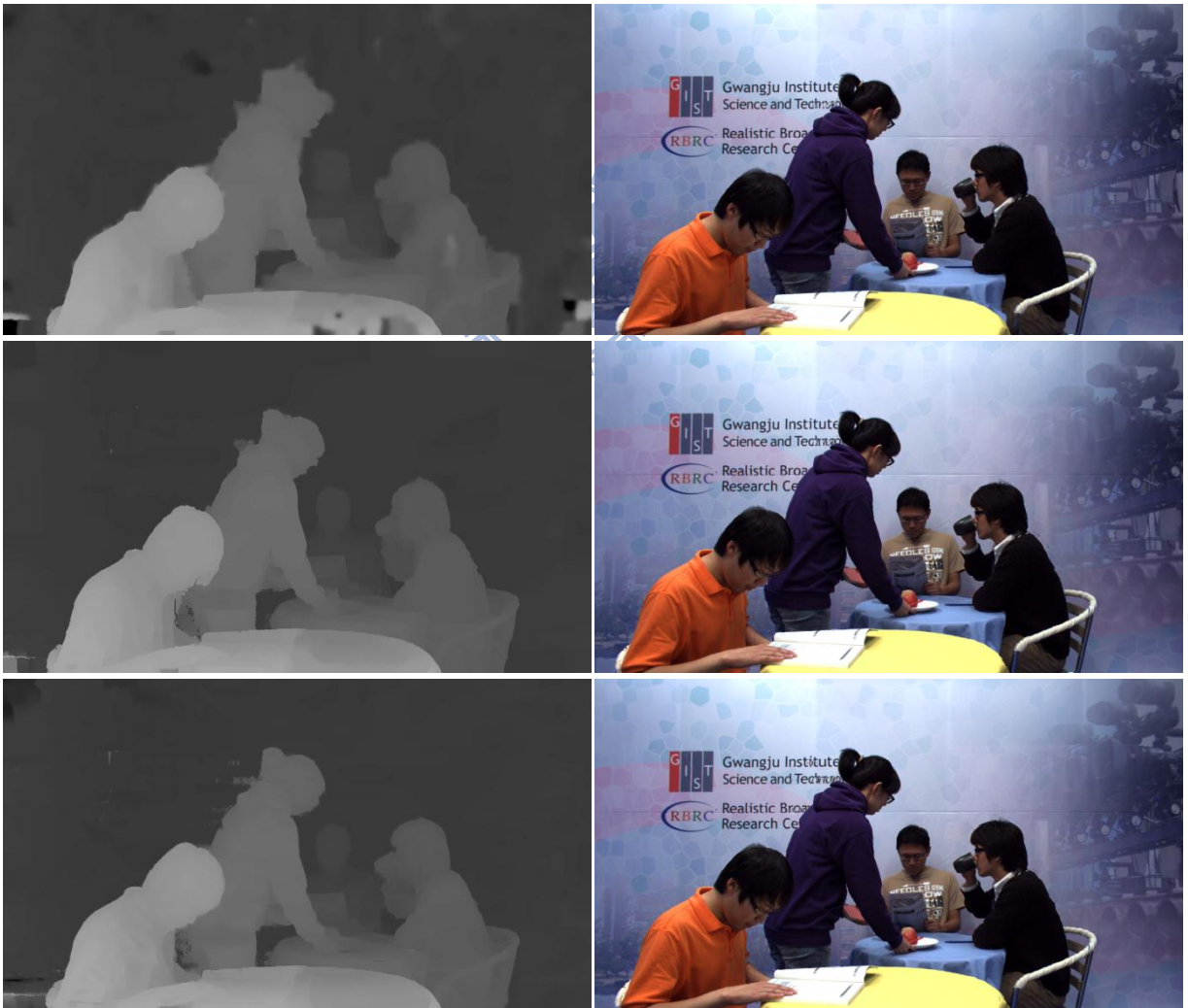
Figure V-8 Disparity maps and view synthesized images in the 50 th frame of Café Results from top to down are the produced by the baseline, HQ-DE, HE-DE algorithms.
