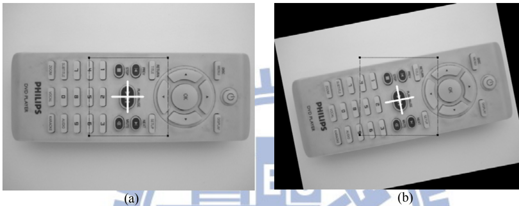
Figure 5-4: (a) Reference image. (b) Testing image with scale=0.9, rotation=-10°, vertical translation=5, horizontal translation=10.
