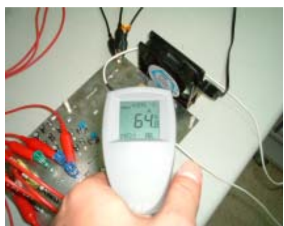
Fig. 4-12 Chip's temperature when power on without fan
