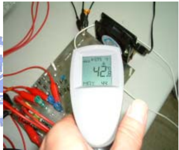
Fig. 4-11 Chip's temperature when power on with fan
