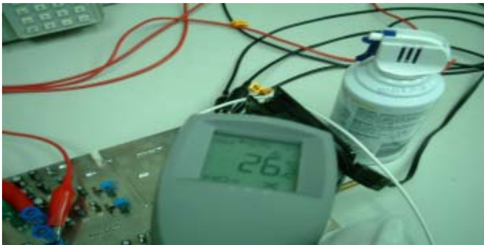
Fig. 4-21 Measured chip's temperature after cooling down the chip 5 seconds
