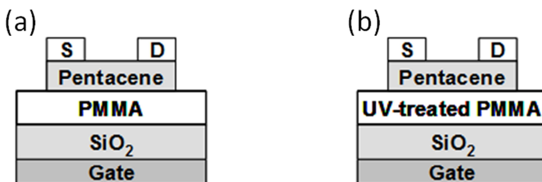
Figure 5.1 Device structure of (a) STD-OTFT and (b) UV-OTFT.
