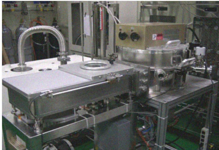
Fig. 22 The figure shows the deposition equipment- 40.68MHz VHF-PECVD.
