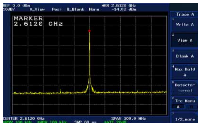
Fig.63 The output power of transmitter
