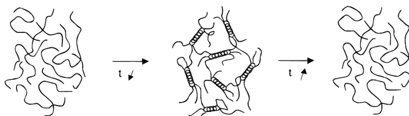
Figure 2.3 Gelatin possesses a triple helix structure at room temperature and forms a stable gels (middle). While increasing above the breaking temperature of hydrogen bonds, the gelatin becomes solution states (right). Copyright 2000, American Chemical Society. [32]
