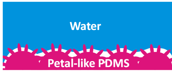
Figure 4.19 Water penetrate the microscale convex and partial wetting the upper part of nanoscale wrinkles.
