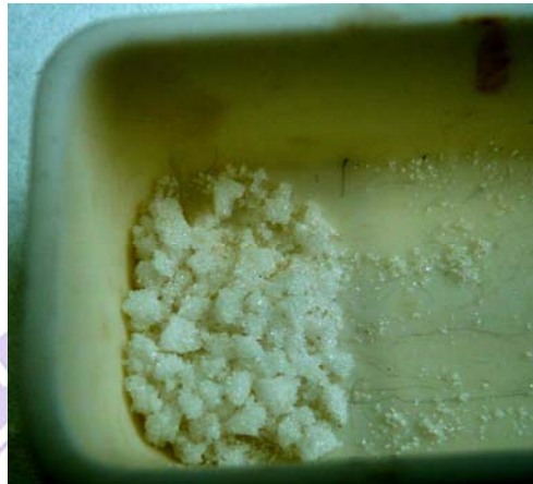
Figure 4.4: Photograph of solid crystalline adamantane powder.
