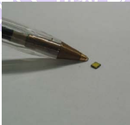
Figure 2.5: Photograph of commercial HPHT diamond (ball point pen for scale).
