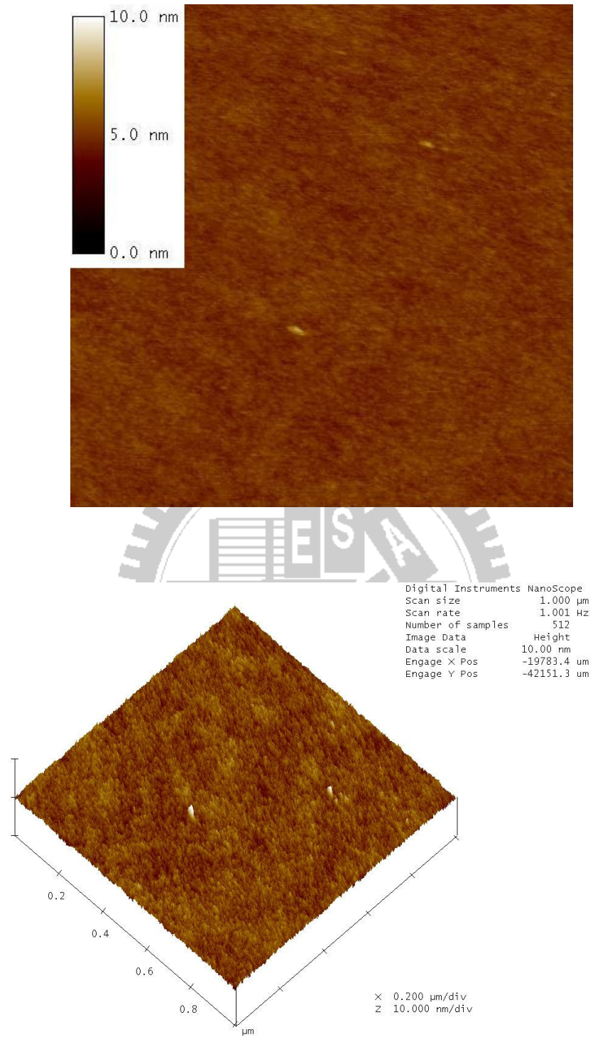
Figure 3.2 SPM images of spin-on NiTiO 3 films with different thermal treatments at 200°C.
