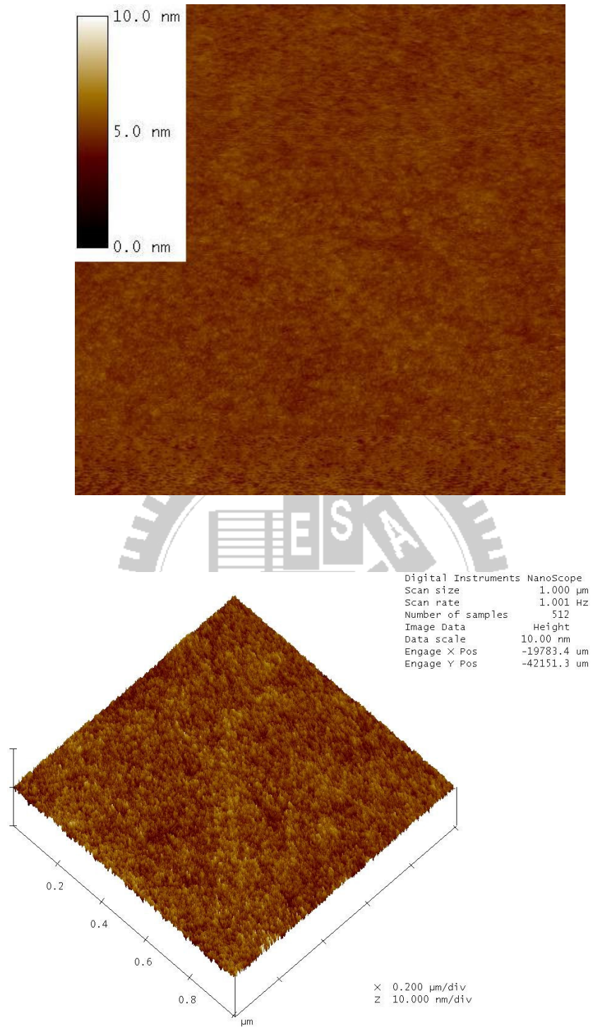
Figure 3.4 SPM images of spin-on NiTiO 3 films with different thermal treatments at 500°C.
