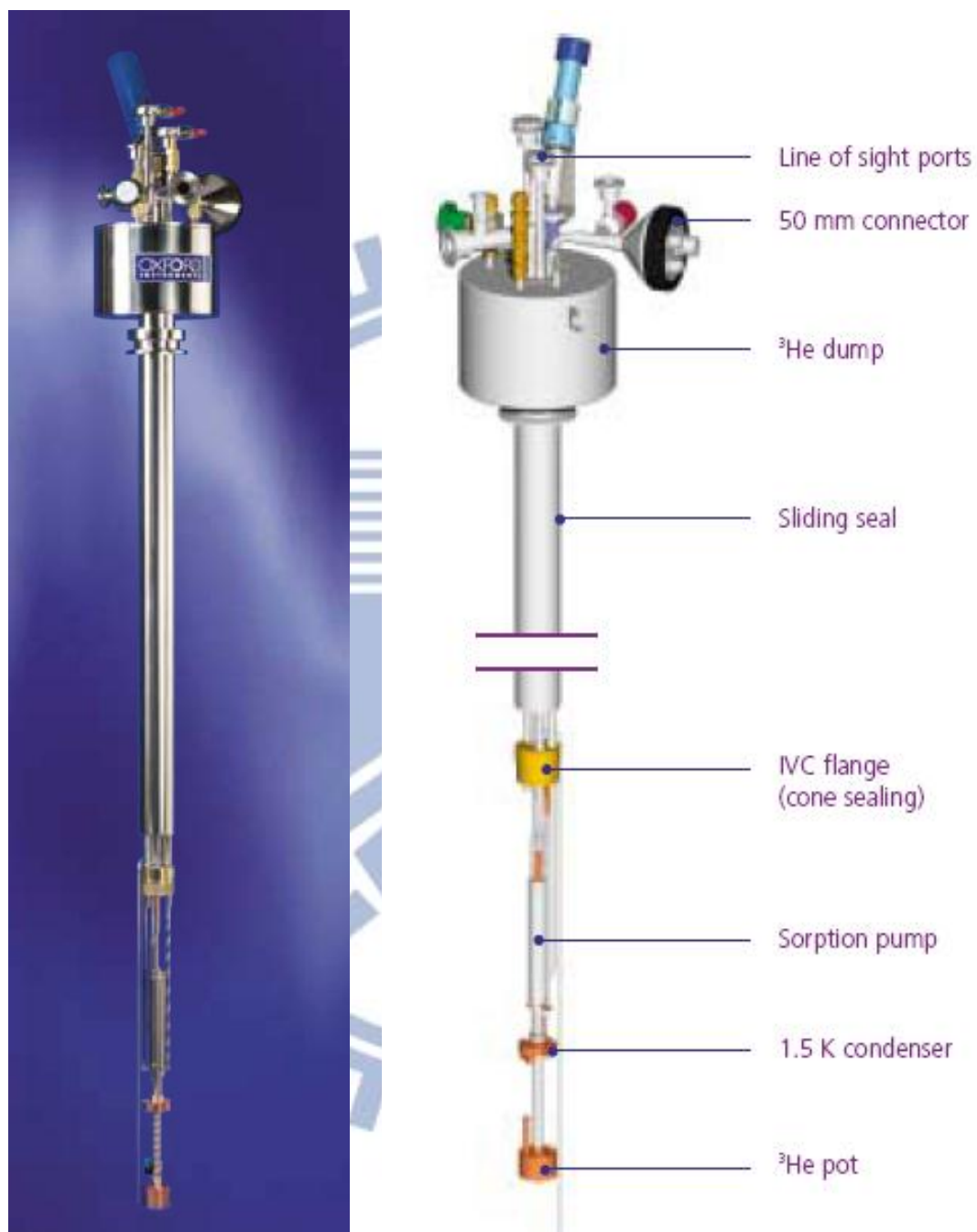
Fig. 3.3 (a) The photo (left) and schematic figure (right) of \text{He}^3 cryostats.
