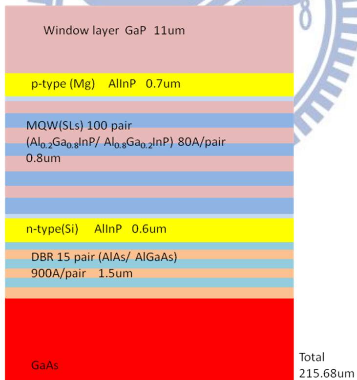
Fig. 3.12 Sample structure of the yellow LED
