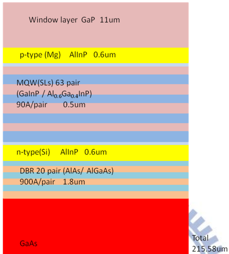
Fig. 3.11 Sample structure of the red LED
