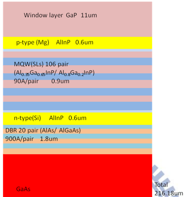
Fig. 3.13 Sample structure of the yellow-green LED
