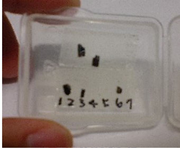
Figure 2-1: The HoMnO 3 single crystals used in this study. The largest surface is around 3 \times 3 mm 2 and the thickness of this crystal is about 0.5 mm
