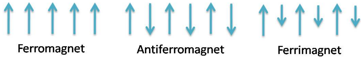
Figure 1-4 Ferromagnetism: (a) Ferromagnetic materials exist a strong coupling between magnetic atoms and the spins align in the same direction even at zero field. (b) An opposite coupled spins in antiferromagnetic materials (NiO, CoO) makes the net moment is zero. (c) Ferrimagnetism such as TbFe and Fe 3 O 4 possesses unequal magnetic moments and hence nonzero moments.
