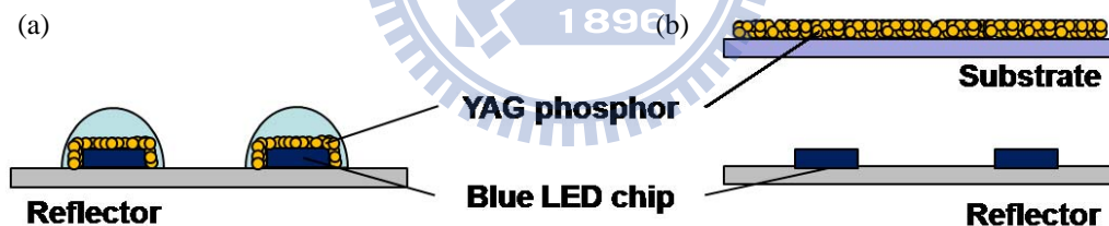
Fig. 5-1. Scheme of (a) conventional direct-emitting backlight using white LEDs and (b) BLPL system.
