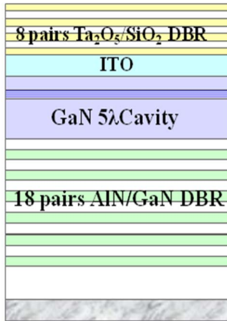
Figure 2. 7 The simulation cavity structure
