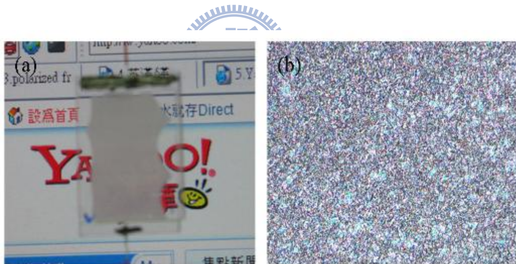
Fig. 6-6 (a) photo and (b) microscopic texture of R3206 in a cell without surface treatment; the cell gap is 5\ \mu\text{m} .
