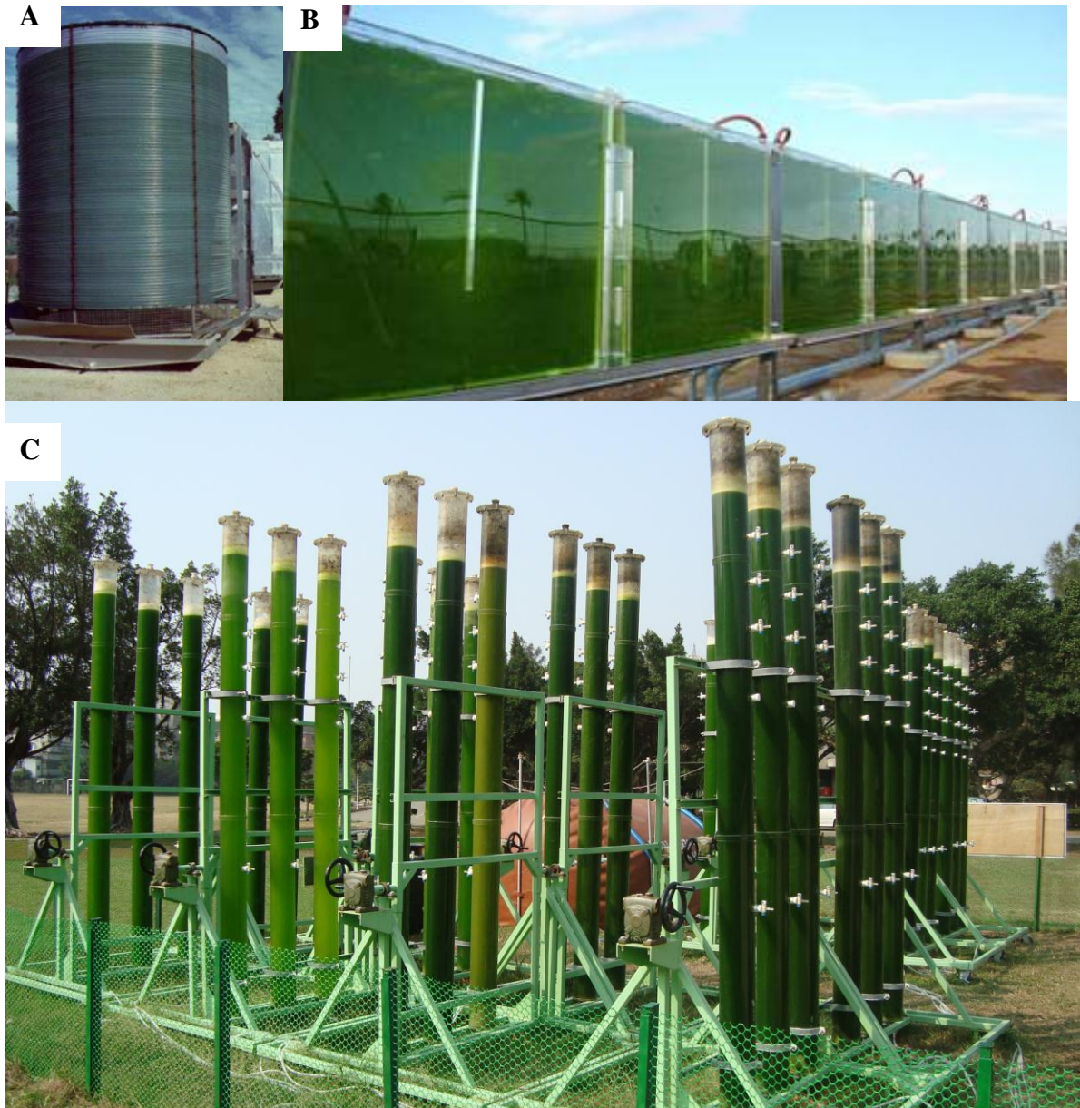
Figure 1. The typical types of photobioreactors. (A) tubular photobioreactor, (B) flat plate photobioreactor and (C) column photobioreactor °
