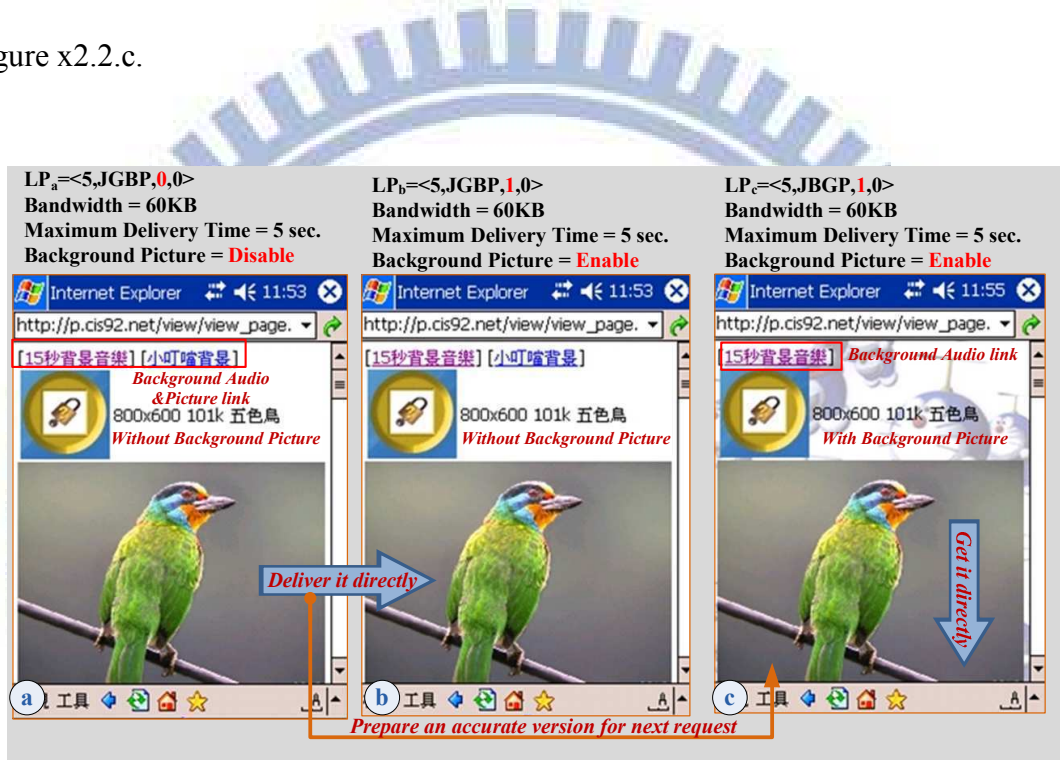
Figure x2.2: (a) Adapted content version of LP_a ; (b) delivered the adapted content version of LP_a for LP_b due to the higher similarity; and (c) delivered the content version created by LP_b in advance for LP_c
