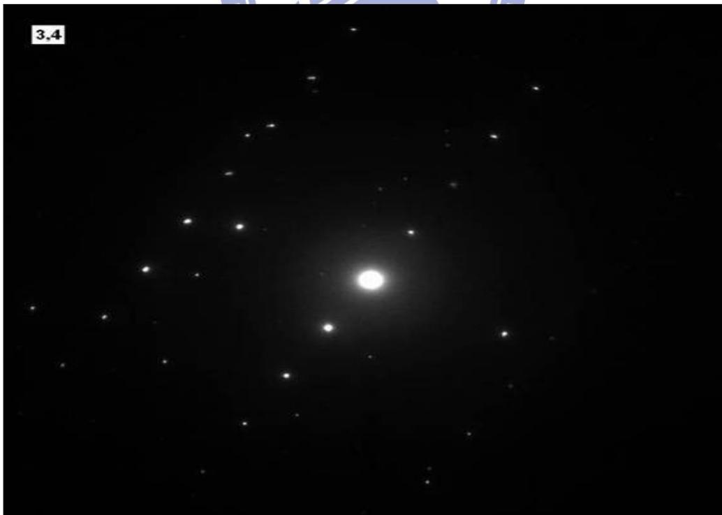
圖 4-25 TEM analysis-SAD Pattern –without O<sub>3</sub> treatment
