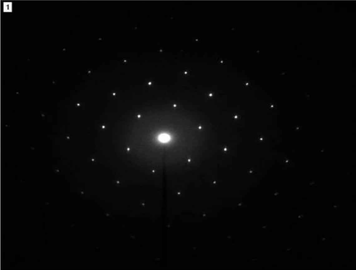
圖 4-33 TEM analysis SAD Pattern-with  $O_3$  treatment
