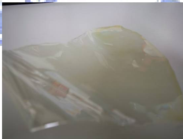
Figure 4.3 The BAPP-ODPA polyimide was tough and useful when an anhydrous DMAc solvent was used.
