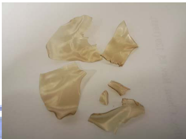
Figure 4.2 The BAPP-ODPA polyimide was brittle when a hydrous DMAc solvent was used.
