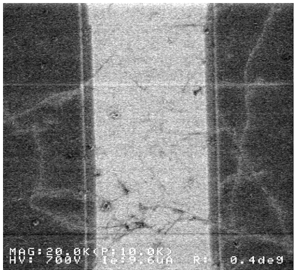
Fig. 4-2. (a) SEM image of CNT coating with over-dense concentration. Large clusters with thousands of CNTs could be observed. (b) SEM image of CNT coating with proper concentration. Only a few CNTs are crossing the channel. No aggregation are observed.
