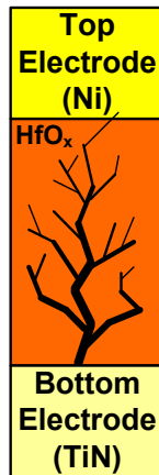
Fig. 1-4 Conductive filament of on state
