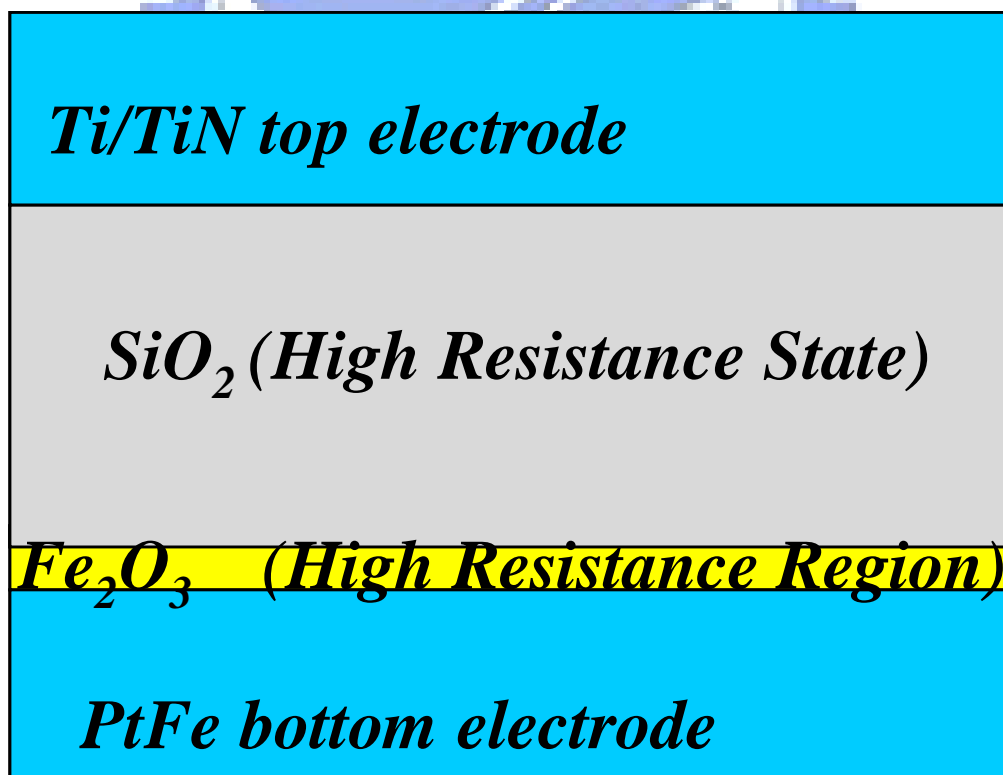
Figure 3.12. Initial state of Al/SiO 2 /PtFe structure.
