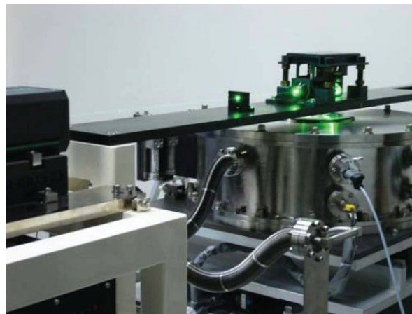
Fig. 2-2 The setup of DPSS continuous-wave laser crystallization.
