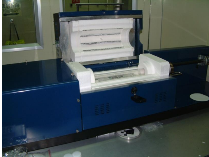
Fig. 2-4 (a) Schematic picture and (b) photograph of thermal CVD.
