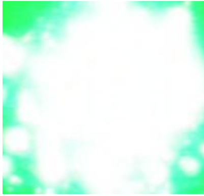
[Fig 3.3.6] Image of fluorescent screen monitoring the field electron emission from the pillar array ( 10\text{mm} \times 10\text{mm} ) at an electric field of 0.66\text{ V}/\mu\text{m} .
