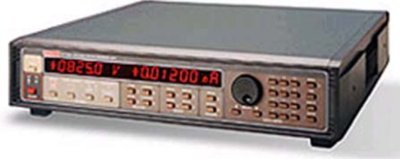
Keithley Model 236 Source-Measure Unit
