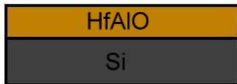
Fig.2-3 (1)Si substrate RCA clean (2)3 nm HfAlO was deposited on the sub-Si by MOCVD.
