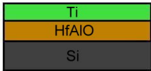
Fig.2-5 20 nm Ti was deposited on the HfAlO layer by dual e-gun evaporation system .
