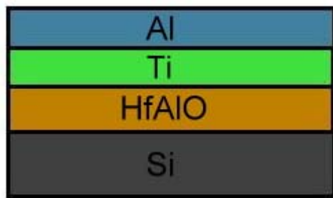
Fig.2-6 400 nm Al was deposited on the Ti layer as top electrode by dual e-gun evaporation system.
