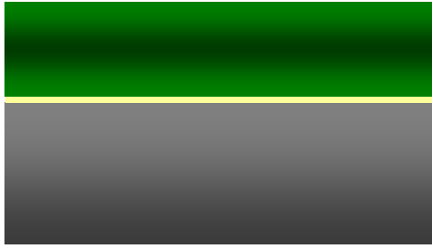
Fig. 2.1 (a) Deposition of 200 nm un-doped poly-Si layer after forming the 3 nm gate oxide with thermal oxidation.
