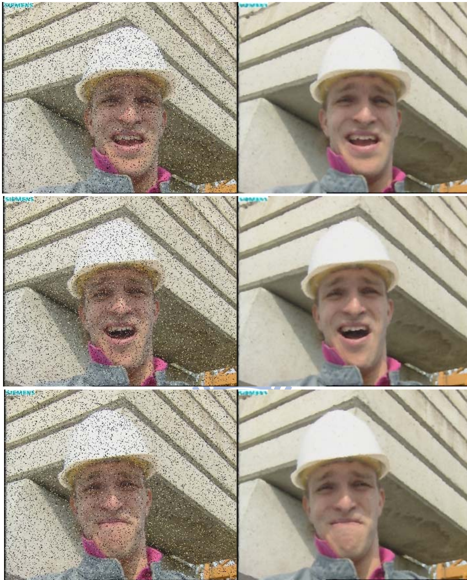
Figure 4-8 The impulse noise reduction results for video frames ( p = 15\% for gray channel)
