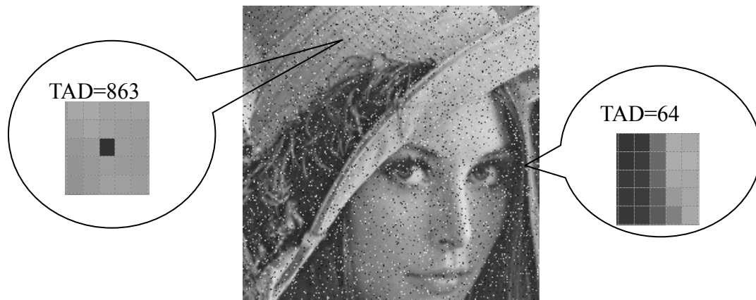
Figure 3-8 An impulse noise pixel (upper side) and a typical edge pixel (right side). TAD of impulse = 863; TAD of edge pixel = 88
