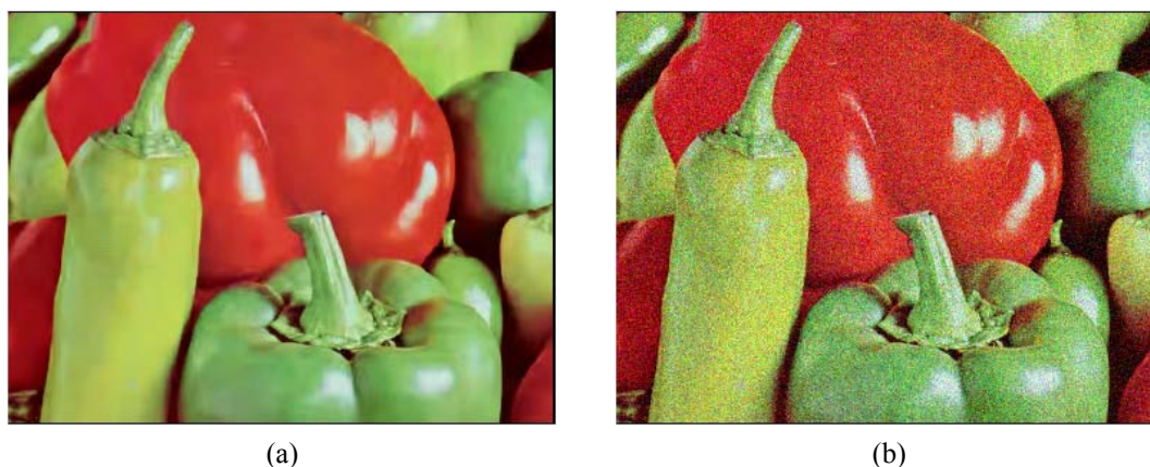
Figure 2-1 (a) The pure image and (b) the degraded image with additive Gaussian noise
