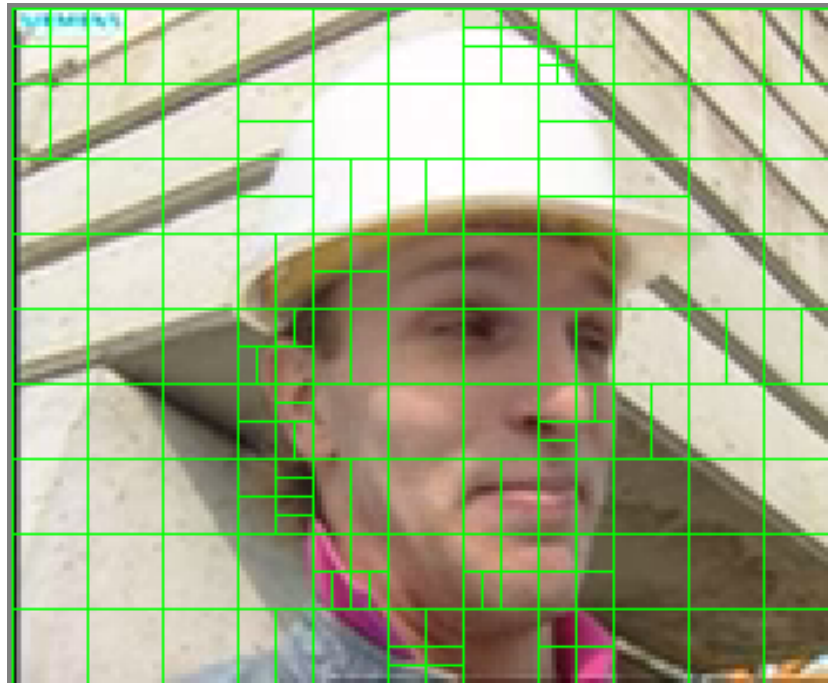
Fig. 4.1. Variable block size in inter-coded block
