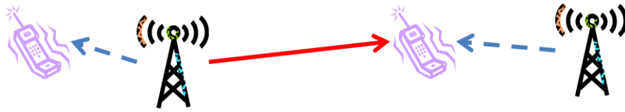
Figure 6 An example of two femtocells environment with one user significantly interfered.
