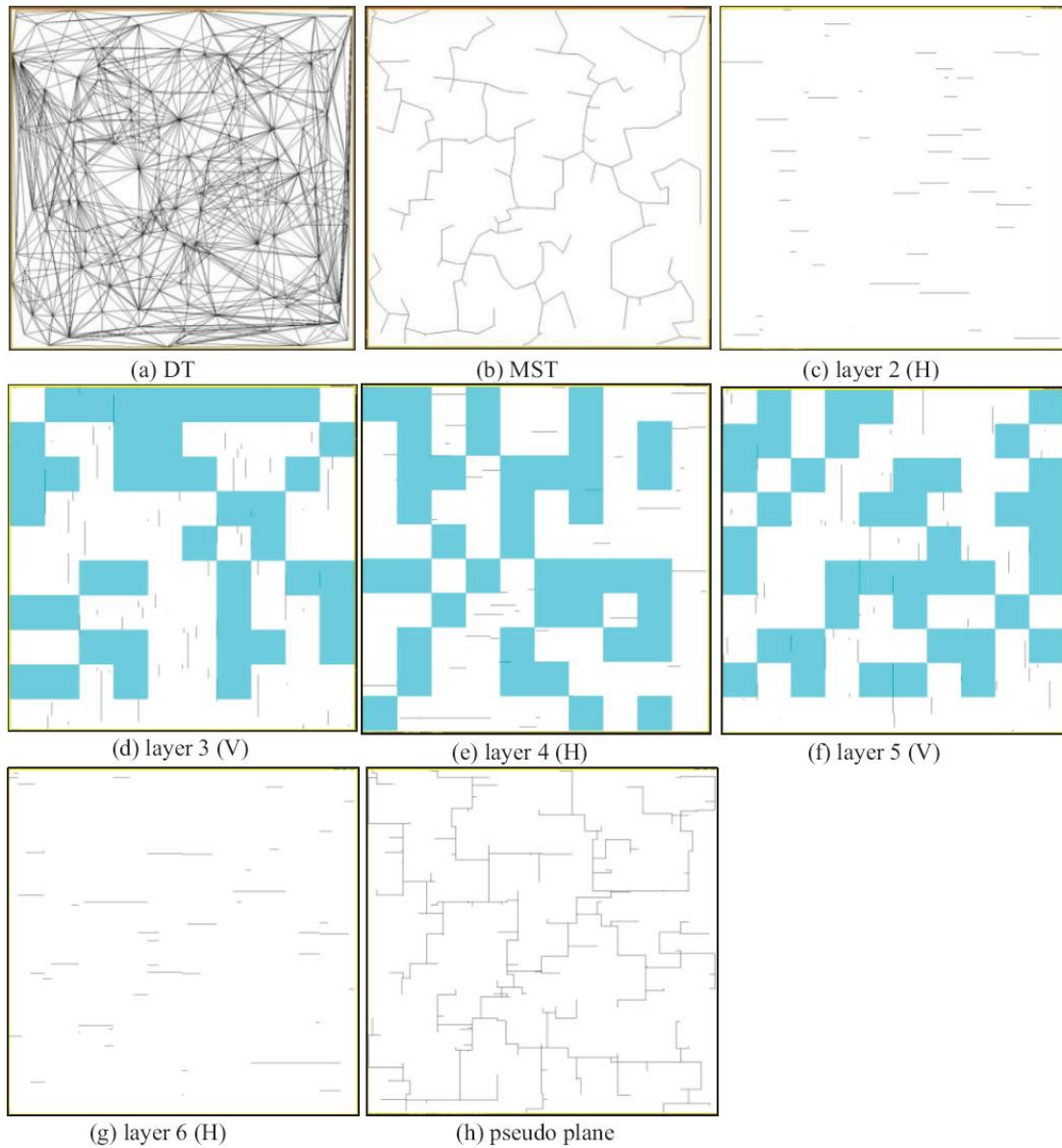
Fig. 15. The OAPDST of ml-ind2 under C_v = 3 . (a) The DT with illegal edges. (b) The MST. (c)-(g) Layers 2-6, respectively. The odd (even) layers allow vertical (horizontal) edges. Some line segments are at obstacle boundaries; they are feasible according to the problem formulation. (h) All pin-vertices are projected onto a pseudo plane, without showing the obstacles.
