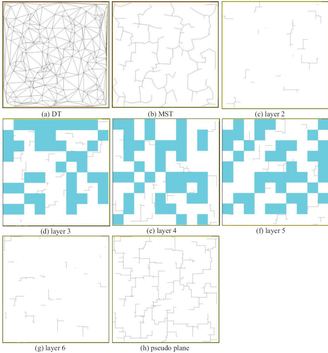
Fig. 14. The ML-OARSMT of ml-ind2 under C_v = 3 . (a) The DT without illegal edges. (b) The MST. (c)-(g) Layers 2-6, respectively. (h) All pin-vertices are projected onto a pseudo plane, without showing the obstacles.
