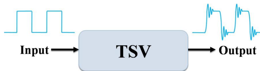
Figure 2.6: A block diagram of a clock signal passes through a TSV
