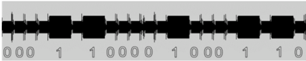
Figure 4.1: The power trace of a straightforward RSA implementation.
