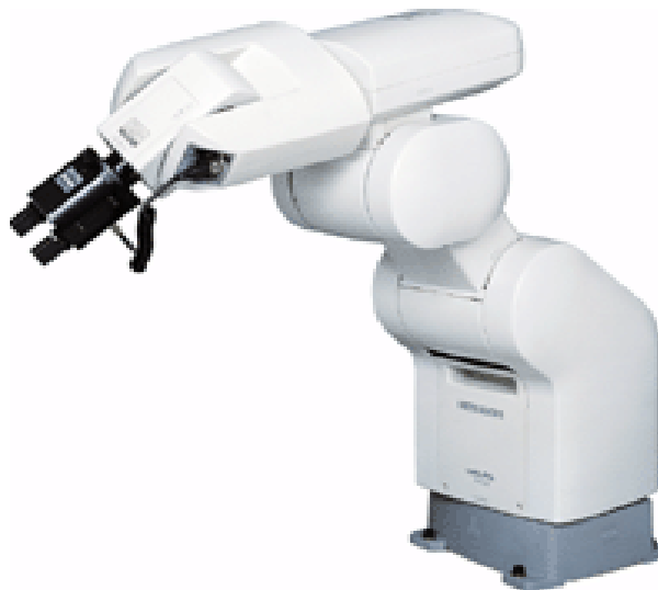
Fig. 3.9: Mitsubishi RV-2A type vertical six-axis robot arm
