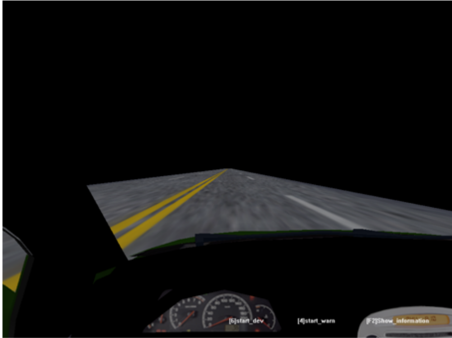
Fig. 2-3: The overview of surrounded VR scene. The VR-based highway scenes are projected into surround screen with seven projectors.
