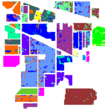
Figure 2. The support vector machine (SVM) classification results of the Indian Pine Site image, containing speckle-like errors.
